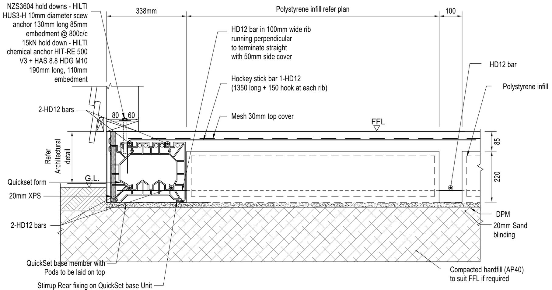
**QUICKSET TIMBER WEATHER BOARD PERIMETER DETAIL**
