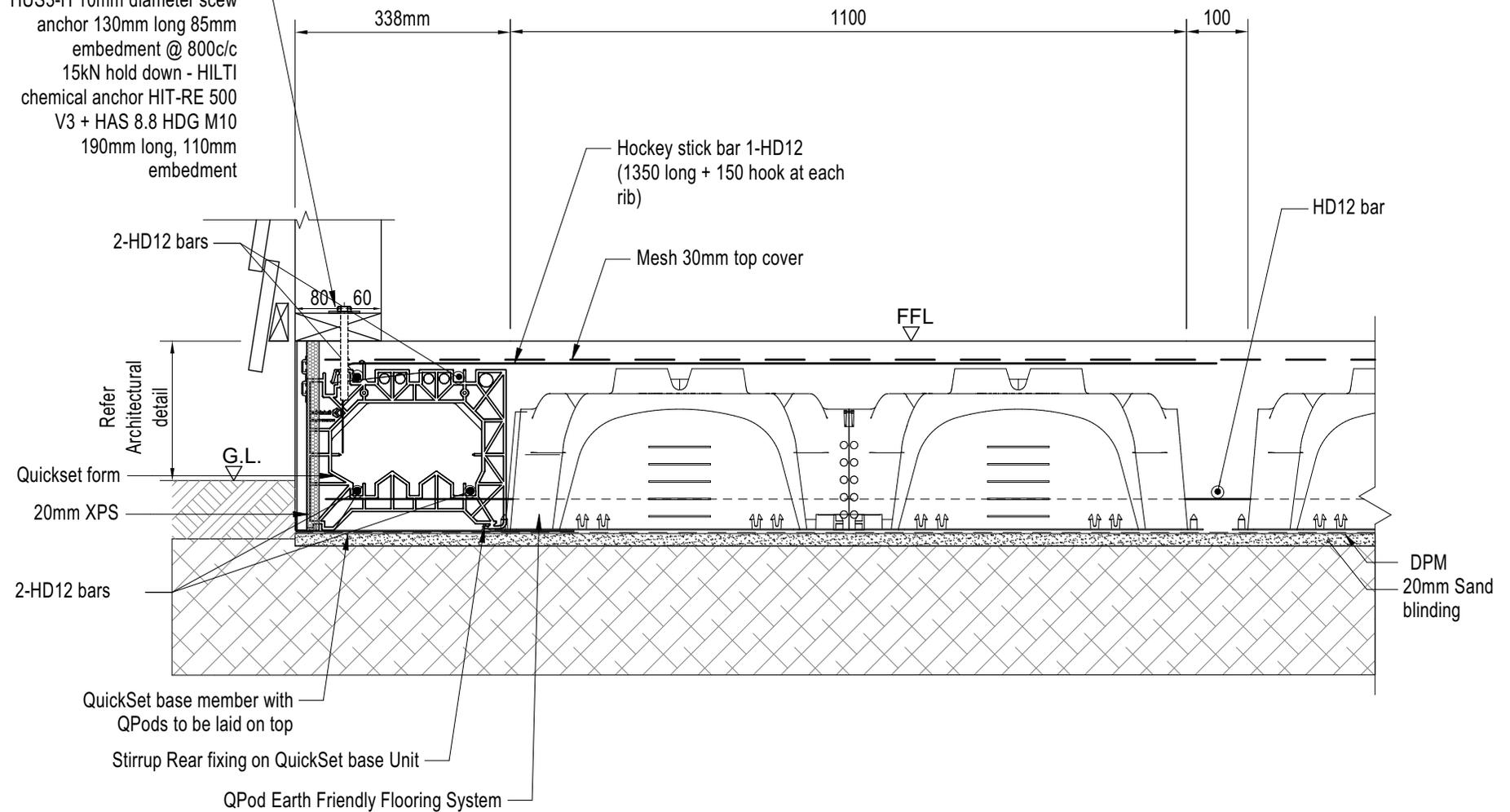
**QUICKSET TIMBER WEATHER BOARD QPod PERIMETER DETAIL**
