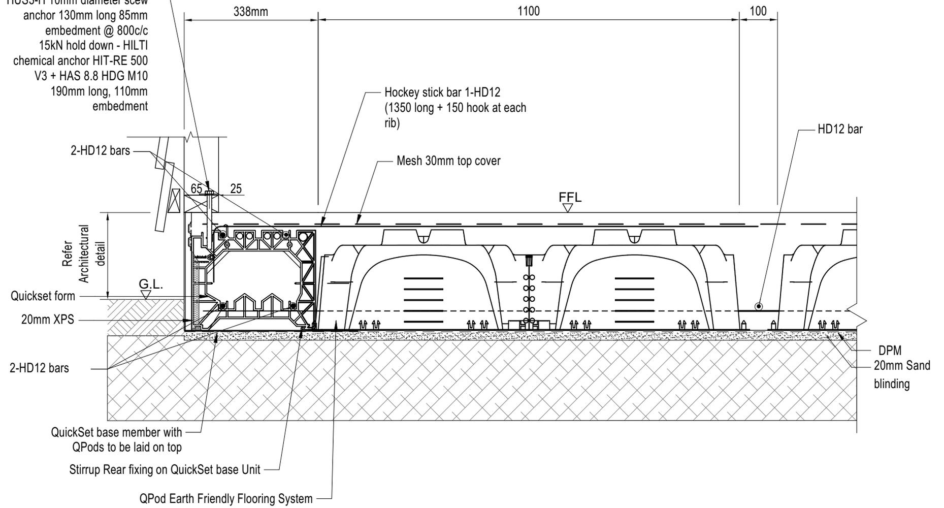
**QUICKSET TIMBER WEATHER BOARD QPod PERIMETER DETAIL**
