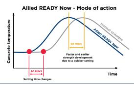
Please note that this concrete will still be susceptible to damage if it is placed upon frozen ground and it is not to be considered as a material exempt from the precautions listed in Section C7.2.1 and C7.2.2 of NZS 3109.
