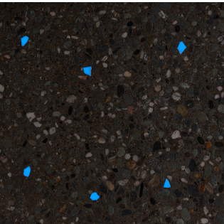
500mm x 500mm sample with a dose equivalent to 100g/m².
